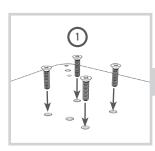
4 FLAT HEAD SCREWS SCREW THROUGH TOP PLATE IN 4 HOLES THAT FORM A "SQUARE" AND INTO THE COLUMN. MAKE SURE SCREWS ARE FLUSH.
