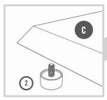
SCREW 4 LEVELERS INTO INSERT SLOTS ON BOTTOM OF BASE.
